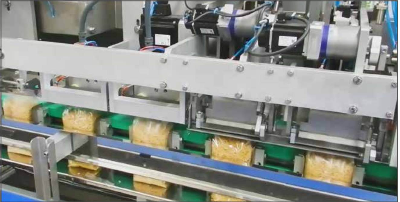
The new MCRS-VD packaging system enables the packaging of up to 180 packs of pasta per minute.
