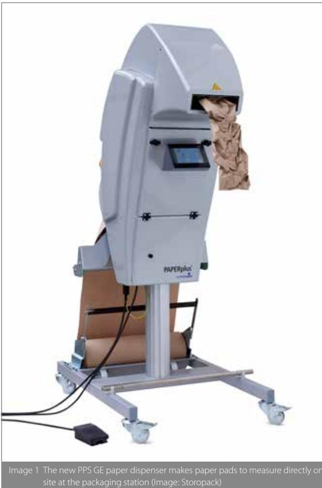
Image 1 The new PPS GE paper dispenser makes paper pads to measure directly on site at the packaging station (Image: Storopack)
