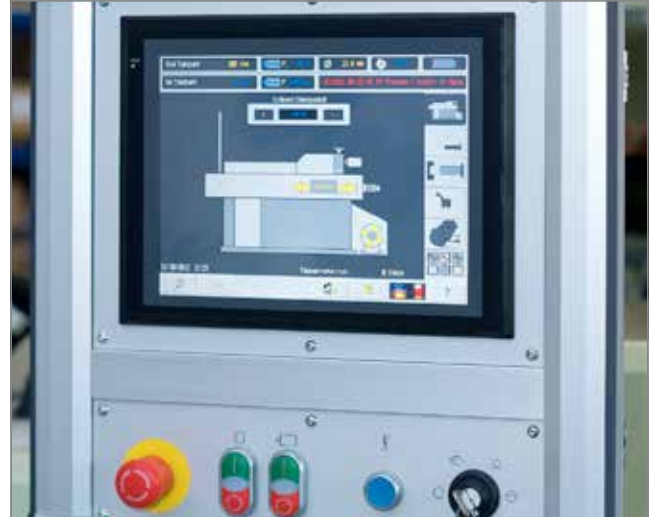
Image 6a,b: Intuitive HMI control panels with 5" and 12" monitors provide clear, easy-to-understand information
