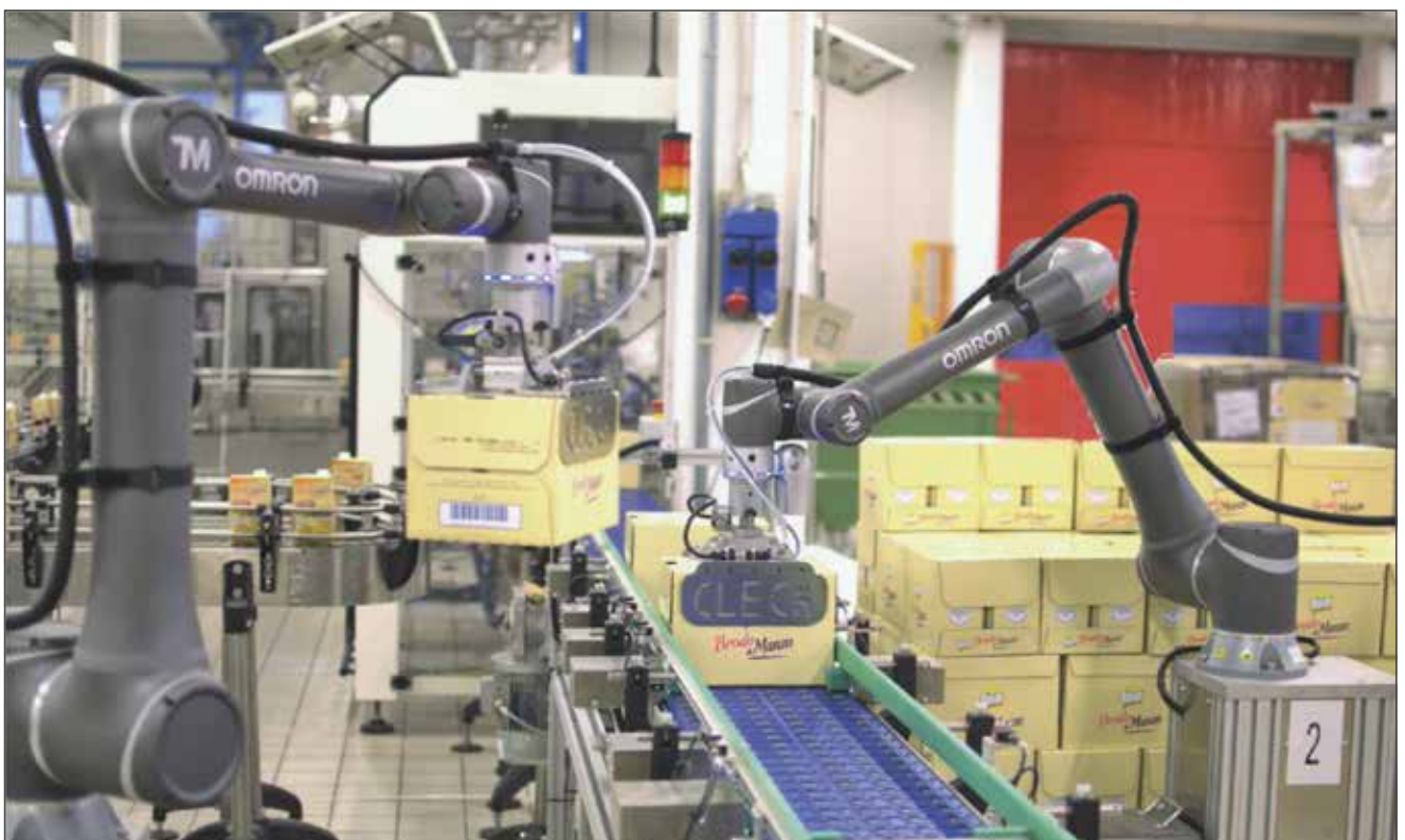
Automation using Omron's TM12 cobots, with a payload of 12Kg and reach of 1,300mm, has enabled the company to achieve its objectives.
