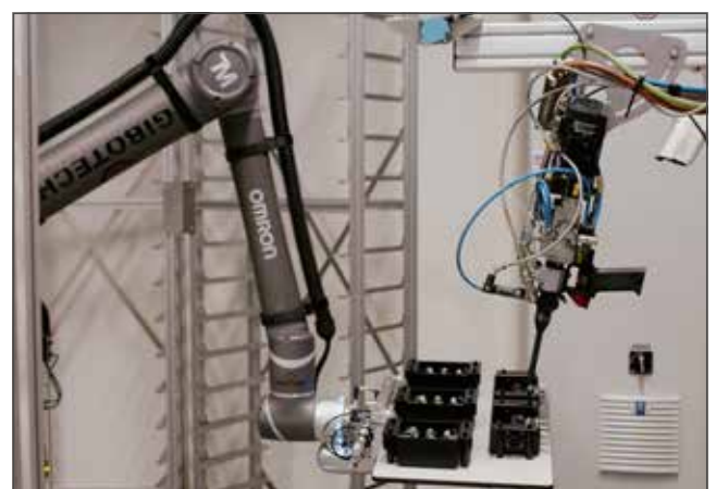
The cobot collects the tray and moves it so that it's underneath an epoxy extruder.
