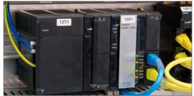
Image 3 The pouch cutter is controlled by the future-proof NJ3-1200 machine controller of the Sysmac automation platform.
