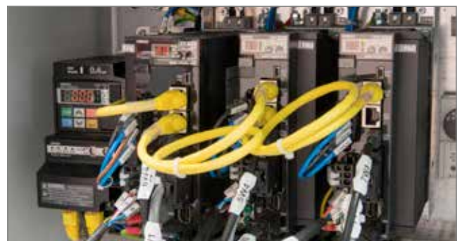
Image 4 Three servo drives are used to position the continuous web, drive the rotating cutting edge, and ensure synchronous transfer to the downstream machine.
