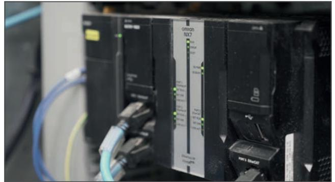
*In addition to the five AMRs, OMRON also supplied the Sysmac machine controller.*
