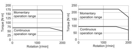
Note The continuous operation range is the range in which continuous operation is possible at an ambient temperature of 40°C when the Servomotor is horizontally installed on a specified radiator plate.
