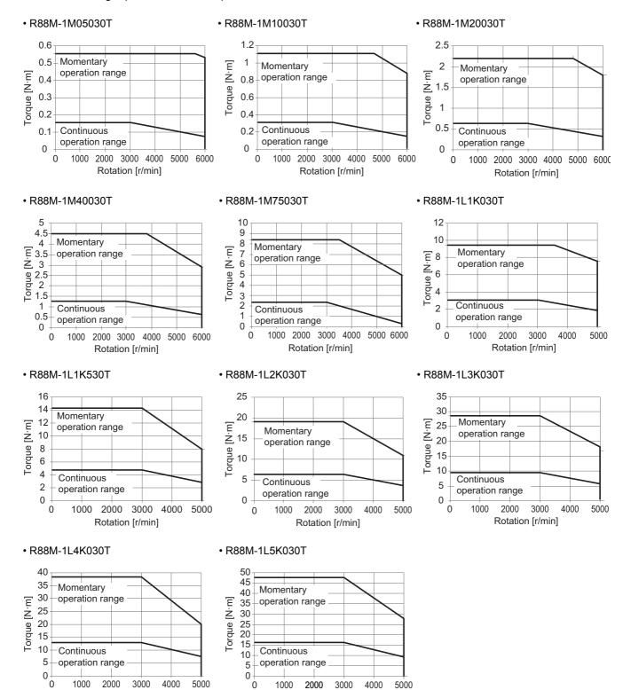
Note The continuous operation range is the range in which continuous operation is possible at an ambient temperature of 40°C when the Servomotor is horizontally installed on a specified radiator plate.
