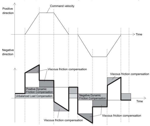
Note The dynamic friction compensation holds the compensation value until the command direction changes, in order to sustain the position during stabilization.
