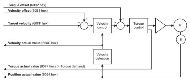
The following diagram shows the configuration of the control function of the Cyclic synchronous velocity mode.
