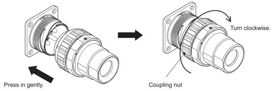
When fitting is completed, the arrow marks of the plug and receptacle are aligned.
