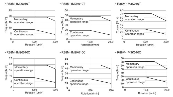
Note The continuous operation range is the range in which continuous operation is possible at an ambient temperature of 40°C when the Servomotor is horizontally installed on a specified radiator plate.
