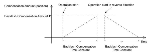
To determine the actual position of the Servomotor, the Servomotor position data acquired via Ether-CAT communications is offset by the Backlash Compensation Amount.
