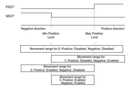
Note that the Servomotor does not stop if **Max Position Limit** (3B11-04 hex) is equal to or smaller than Min Position Limit (3B11-03 hex).
