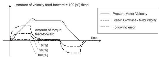
You can reduce the following error in a constant acceleration range by using the torque feed-forward.
