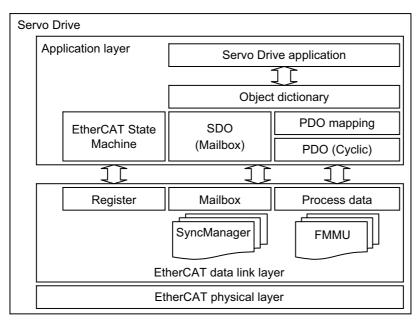
Normally, EtherCAT can transmit different protocols. 1S-series Servo Drives with Built-in EtherCAT Communications use the IEC 61800-7 (CiA 402) drive profile.
