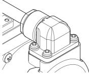
Note Make sure that the connector is securely fitted into place without a gap or tilt. Do not tighten the screws if the connector is not securely fitted into place. Doing so may result in a damage. Tighten the four screws evenly.
