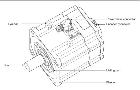
200 VAC 4 kW Servomotors (with Brake)
