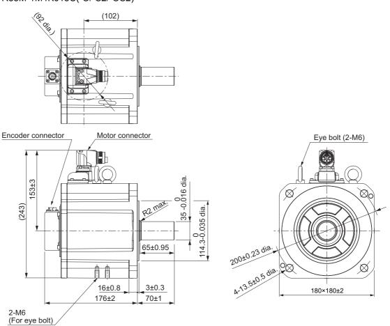
Note The standard shaft type is a straight shaft. Models with a key and tap are indicated with "S2" at the end of the model number.
