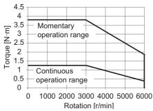
Note The continuous operation range is the range in which continuous operation is possible at an ambient temperature of 40°C when the Servomotor is horizontally installed on a specified radiator plate. Continuous operation at the maximum speed is also possible. However, doing so will reduce the output torque.
