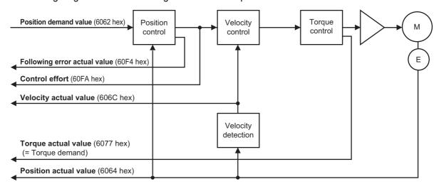
The following diagram shows the control function configuration of Profile position mode.
