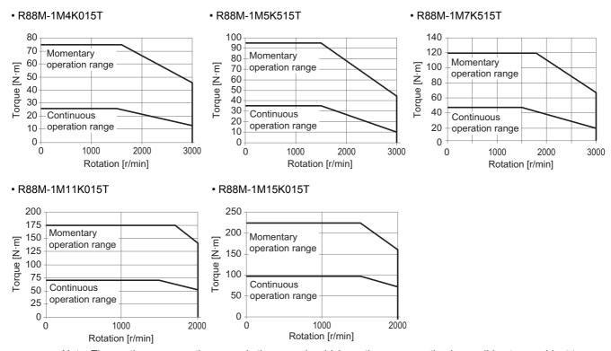
Note The continuous operation range is the range in which continuous operation is possible at an ambient temperature of 40°C when the Servomotor is horizontally installed on a specified radiator plate. Continuous operation at the maximum speed is also possible. However, doing so will reduce the output torque.
