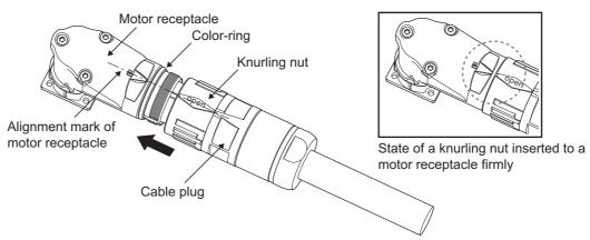
4 Turn the knurling nut to clockwise direction until it stops.
