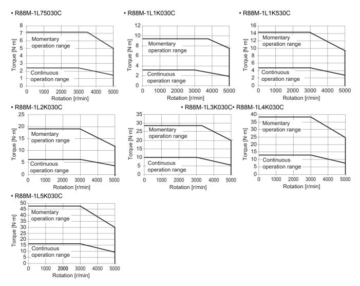
Note The continuous operation range is the range in which continuous operation is possible at an ambient temperature of 40°C when the Servomotor is horizontally installed on a specified radiator plate. Continuous operation at the maximum speed is also possible. However, doing so will reduce the output torque.
