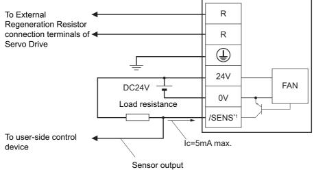
\*1. Build a system to prevent the Servomotor from operating if a fan error is detected by the /SENS signal.
