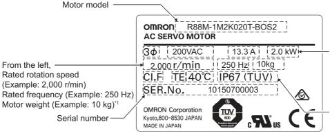
\*1. The weight is not given for the Servomotor with a flange size of 80 x 80 or less.
