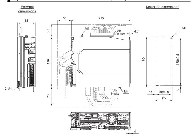
Single-phase/3-phase 200 VAC: R88D-1SN15H-ECT (1.5 kW) 3-phase 200 VAC: R88D-1SN20H-ECT/-1SN30H-ECT (2 to 3 kW) 3-phase 400 VAC: R88D-1SN06F-ECT/-1SN10F-ECT/
