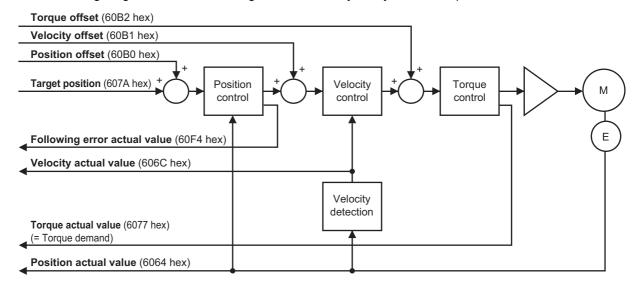
The following diagram shows the configuration of the control function of the Cyclic synchronous position mode.
