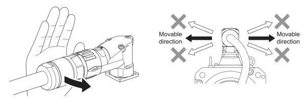
Use your hand, instead of tool, etc. when changing the cable outlet direction. Otherwise, a large amount of force is applied easily even toward not-specified direction and may cause failure of the connector.
