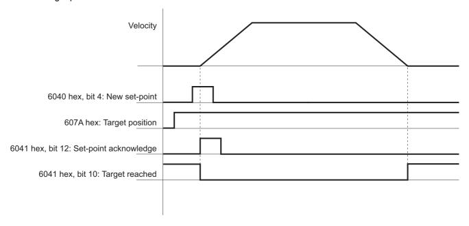
You can change the target value while PTP positioning is in progress.
