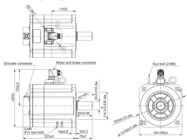
Note The standard shaft type is a straight shaft. Models with a key and tap are indicated with "S2" at the end of the model number.
