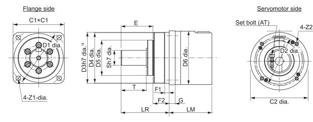
Key and tap dimensions \*4. The tolerance is "h8" for R88G-HPG50 $\square$ .
