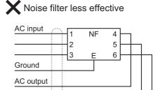
• The power cables must be twisted or tightly bundled.
