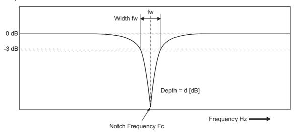
If mechanical resonance occurs, use this notch filter to eliminate resonance.
