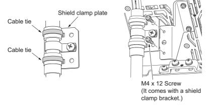
Do not put loads on the cable and the shield clamp such as twisting, pushing and pulling, etc.
