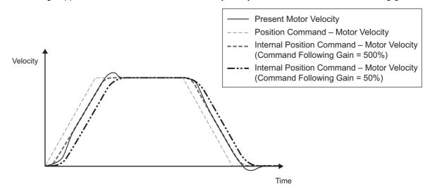
The smaller the set value of Command Following Gain is, the more the overshooting can be suppressed.
