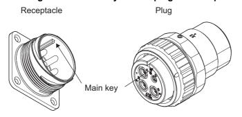
\* The arrow mark on the receptacle shell indicates the position of the main key.
