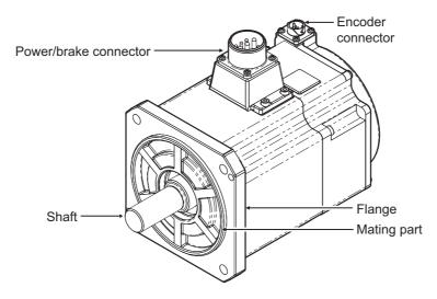
200 VAC 1.5 kW Servomotors (with Brake)
