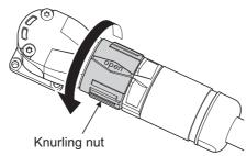
Pull the cable plug out the motor receptacle linearly.
