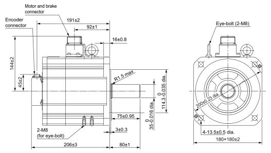
Note The standard shaft type is a straight shaft. Models with a key and tap are indicated with "S2" at the end of the model number.
