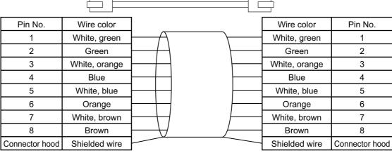
Note 1. Connect the cable shield to the connector hood at both ends of the cable.
