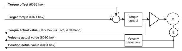
The following diagram shows the configuration of the control function of the Cyclic synchronous torque mode.
