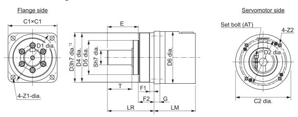
Key and tap dimensions \*3. The tolerance is "h8" for R88G-HPG50  $\square$ .
