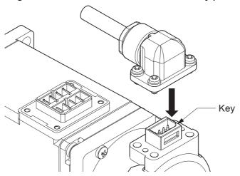
Tighten the screws to fix the connector after it is fitted.
