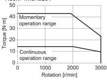
Note The continuous operation range is the range in which continuous operation is possible at an ambient temperature of 40°C when the Servomotor is horizontally installed on a specified radiator plate.
