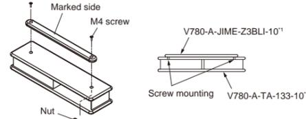
2. Mount the Attachment to which the RF Tag is mounted to the metallic material. Mount it with two M4 bolts. (Recommended tightening torque: 1.2 N·m, M6 bolt mating length: 4 mm min.)
