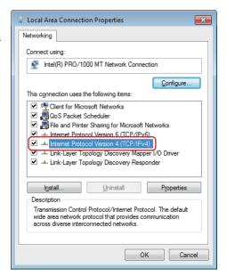
6 Click the [Use the following IP address] option and enter an IP address and subnet mask.
