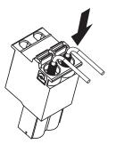
When using single wire, or stranded wire Insert the wire deeply in to the terminal hole while pushing the release button on the side of terminal hole using a screwdriver.
