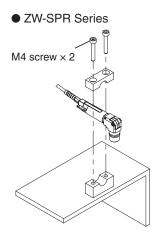
Fix the recommended jig within the shaded area in the figure below.
