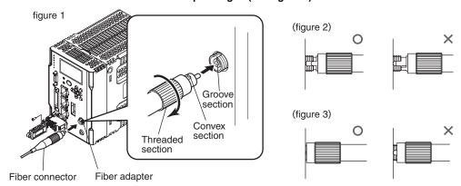
When the fiber insertion/fixing screw is not completely tightened, as is the case in the "No good" status in figure 2 and figure 3, optic signals cannot be transmitted and correct measurement is not possible. Always check that the system is in the "Good" status.
