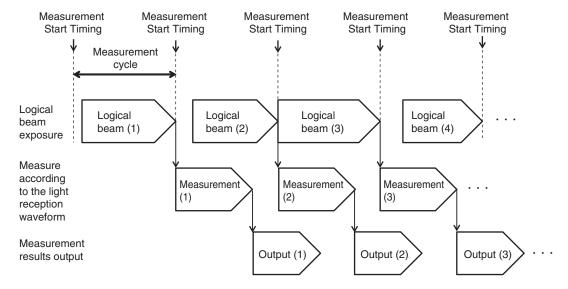
The Sensor Controller starts exposing logical beam when the measurement start timing is specified. When the light power is 100%, exposure starts when the measurement starts, but when the light power is less than 100%, there is a period with no exposure after the measurement starts. The exposure starts when the measurement starts and ends when the measurement cycle ends.
