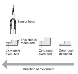
The zero reset function also allows setting the reference value to the hold value for a hold measurement or any value other than zero.
