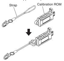
**2** Attach the Calibration ROM to the fiber cable of the Sensor Head.
