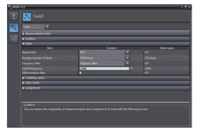
The range of cut-off frequency to be effective in operation varies depending on the setting of measurement cycle.
