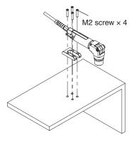
This installation method can be used to install sensor heads next to each other.
