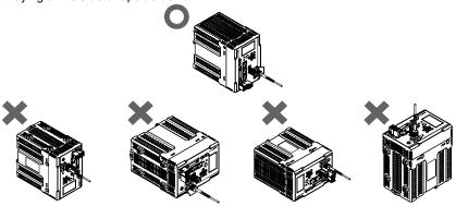
For adequate intake and/or exhaust, keep the Sensor Controller clear by 30 mm or more on its top, and by 10 mm or more from either side.
