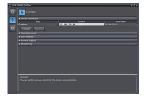
When you click [Connect], the Sensor Controller with the specified IP address is connected. When the connection is successful, Sensor Controller information is displayed.
