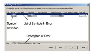
It is now possible to edit the Symbol entries to correct the errors. The new corrections will appear in the 'New?' column or to mark them for deletion.
