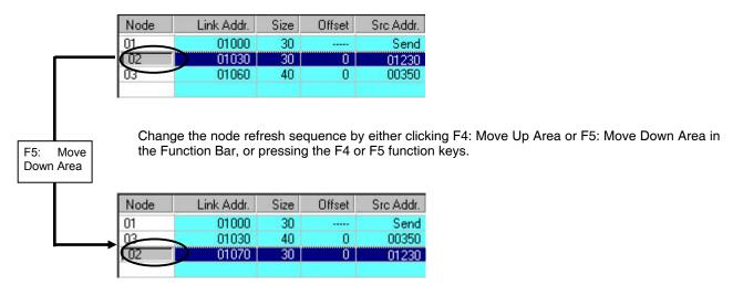
**Reference:** The node refresh sequence for individual nodes cannot be checked in the Data Link Configuration window. Node refresh sequence checking and changes must be performed in the Node Editing window.
