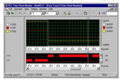
With the CX-Programmer version 6.0 and later versions, data collected by the Data Trace and Time Chart Monitor functions can be saved in standard CSV files (with .csv filename extension). The data saved in standard CSV files can be analysed and printed in programs such as Microsoft Excel.
