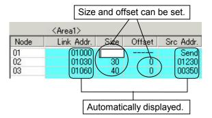
**Reference:** Size modifications and offsets can be set in the Area Specify dialog box that is displayed by double-clicking on the data link configuration icon (oval for send area or rectangular for receive area ).
