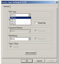
CJ1M-CPU11: Set CPU12.CJ1M-CPU21: Set CPU22.
