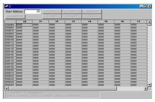
• In the **PLC Memory** window, both individual bits for each word and the hexadecimal value of the word can be monitored at the same time if the display format is set to BIN (binary).
