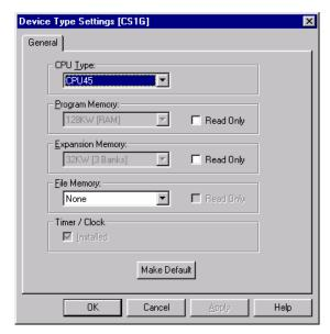
When settings cannot be selected, the PLC is fitted with the standard settings as shown on the Device Type Settings dialog and cannot be reconfigured. Similarly, if Expansion Memory cannot be selected for CV-Series PLCs, EM memory cannot be configured.
