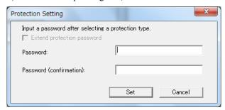
**Note:** If the *Extend protection password* check box is selected, the passwords must contain a maximum of 16 alphanumeric characters. If the *Extend protection password* check box is not selected or not displayed, the passwords must contain a maximum of 8 alphanumeric characters.
