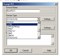
2. Click the **Settings** Button by the *Device Type* Field and set the *CPU Type* in the Device Type Settings Dialog Box as shown below.
