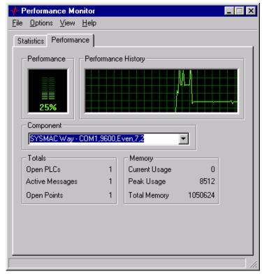
The *Performance* tab displays an automated performance history and performance load for the selected active connection in the *Component* option or for the overall performance. Details of activity are described in terms of the number of open PLCs, active messages and open points in the *Totals* field.
