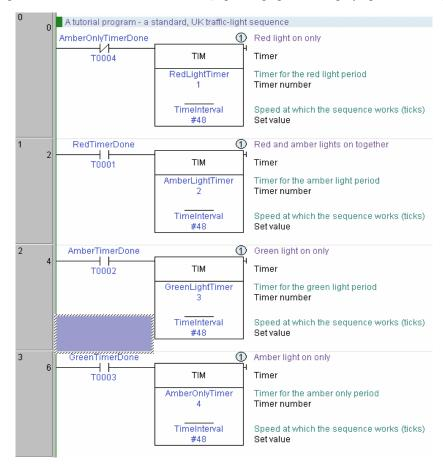
Use the following procedure to place an output for each of the traffic lights into the program.
