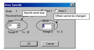
**Note:** With SYSMAC LINK, the send size can be set, but the receive size and the reception offset cannot. Therefore, the Area Specify dialog boxes are as shown in the following example diagrams.
