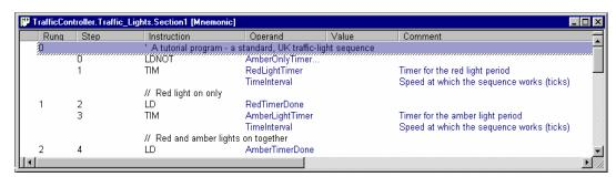
Whenever mnemonic instructions are entered, the Ladder program of the program is updated. When a complete rung has been formed by the entered mnemonics, CX-Programmer normalizes the new mnemonics and redraws the rung.
