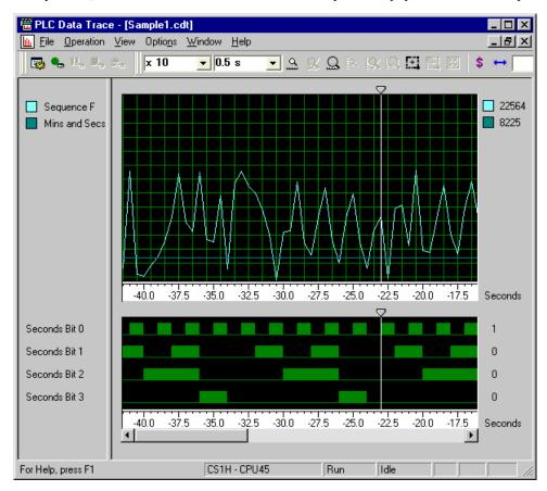
The top graph illustrates the word addresses or symbols. The bottom graph illustrates the bit addresses or symbols. Each word address is colour coded. The word and bit addresses are listed in the left pane; the splitter bar can be
