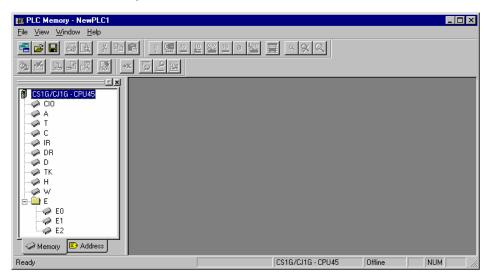
The left pane, known as the Data Area Workspace, displays the current PLC in terms of its data areas and addresses. The data areas that form part of the PLC memory differ depending on the PLC type. The status bar provides instant help, displays the PLC and CPU type and describes the operating mode of the PLC.
