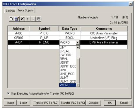
2 Input trace object. The methods of trace object input are the three of the following. Input trace object with the combination of 1ch data, 2ch data, 4ch data, and bit.
