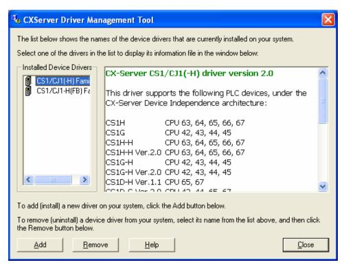
A list of available drivers will be shown on the left pane of the main window. The list is generated when the Driver Management Tool is first opened, and obtained by performing a scan of your computer. When drivers are found, they are shown on the left pane, and once selected, the information about the selected driver is shown in the right pane.
