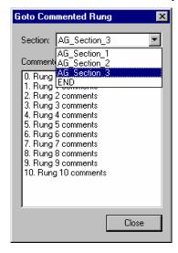
When a rung is chosen, the program section is immediately shown at the chosen position.
