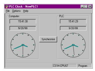
The PLC Clock tool displays two clock images that represent the time for the computer (PC) on the left and the PLC on the right. The time and date are also represented in a digital format for both the computer and the PLC.
