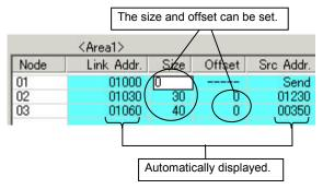
With node address 01, the node refresh sequence matches the default (order of addresses), so no change is required.
