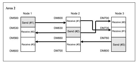
The refresh sequence for nodes 1 and 2 is as follows: #1, #2, #3. For node 3, the order is #2, #1, #3. Node address 03 does not receive all of the data sent from node address 02. Rather, data from the 20 words (CIO 1240 to CIO 1259) beginning from the start address +10 words (i.e., the offset) is received in IR 300 to IR 319. Other data is received with no offset.
