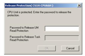
To clear the protection, enter the UM read protection or task read protection password for the current CPU unit, and then click the OK Button. The operation will continue when the protection has been cleared.
