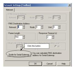
4. The Serial Gateway Guide Dialog Box will be displayed. Select the unit and the port number under the *Calculate Address Area*.
