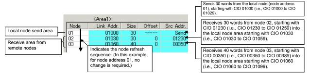
**Reference:** With node address 01, the node refresh sequence matches the default (order of addresses), so no change is required.
