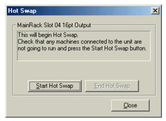
**Note:** Online replacement is possible for a CS1D or CVM1D CPU Unit in any operating mode.
