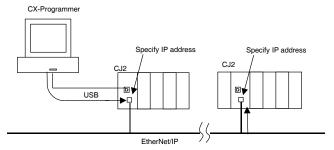
• Connect to the EtherNet/IP network using an Ethernet cable, and connect to the PLC through the network.
