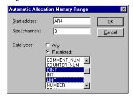
Enter the Start Address, the Size in channels (16 bit words) then select the Data types that can be allocated in that area. On pressing the **OK** button, the address range is checked for validity and an appropriate error message in a message box is displayed. On closing the message box the user is returned to this dialog and the first field that is considered to be in error.
