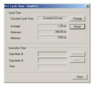
The minimum cycle time and the **Change** Button are displayed only for CJ2H CPU Units with unit version 1.1 or later or CJ2M CPU Units.
