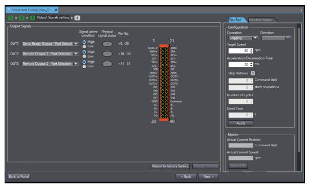
Set the function assignment and monitor the current status of external outputs from the Drive.
