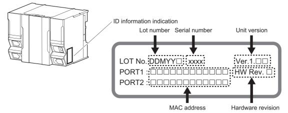
Note The hardware revision is not displayed for the Unit that the hardware revision is in blank. The ID information on an NJ-series NJ501- $\Box$   $\Box$   $\Box$  CPU Unit is shown below.
