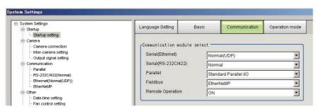
3 Select one of the following Communications Modules based on the communications method that is used to connect with the Sensor Controller and the Unit to connect to, then click [Apply].
