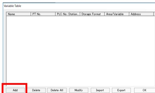
3. Variable Setting dialog box is displayed. Set a variable name, an address corresponding to the variable, data type, and data format.
