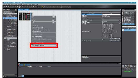
**4** In the device registration area, select the port to connect the IO-Link device to. Then, in the Toolbox, double-click the F39-SGIT-IL3 (Intelligent Tap), or right-click the F39-SGIT-IL3 and select **Insert**. An IO-Link device can also be registered by dragging and dropping it to a port in the device registration area.
