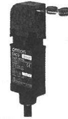
Please keep correct placement between switch body and operation key in mounting so that any excessive force does not apply to the head of the switch body due to out of alignment. Be careful not to deform or damage the operation key by dropping it or by using excessive force to insert it into the switch.
