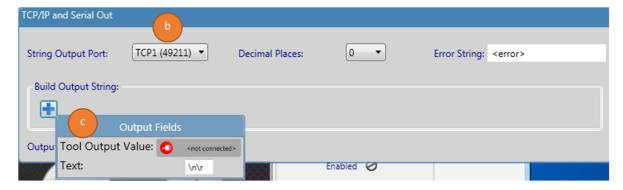
e. Click on the [Not Connected] field, under [Decode1], select [Decoded Text].
