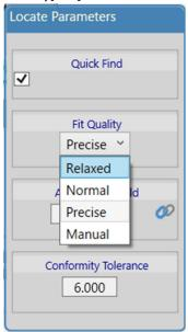
(\*)[Accept Threshold] and [Conformity Tolerance] are automatically set. If part is being located correctly, click [Show Advanced Parameters Window] and adjust other parameters. To check the detail, see HELP.
