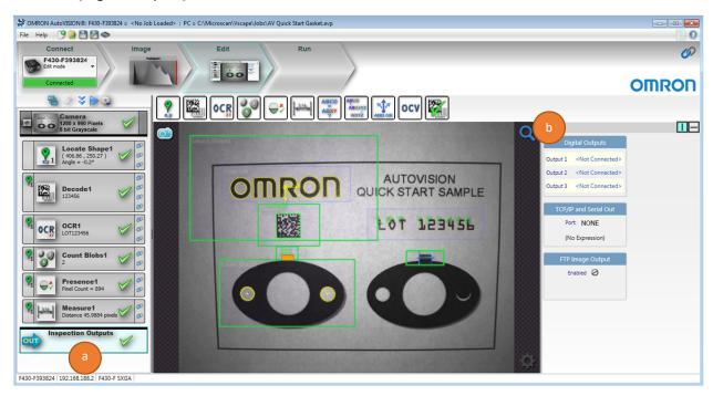
c. Assign the outputs in the Digital Outputs pop up window.
