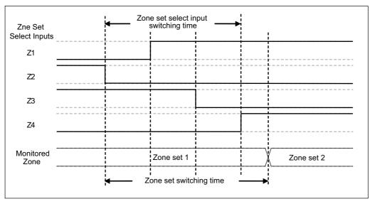
Fig. 2-9 Zone Switching example
