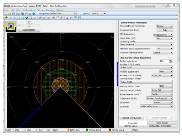
Fig. 3-1 OS32C Configuration Tool
