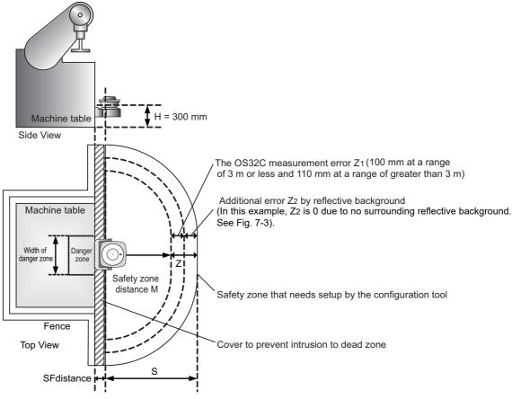
Fig. 4-7 Installation on a Machine
