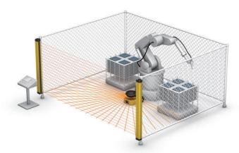
Fig. 1-4 Internal Robot Cell Guarding
