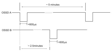
Fig. 2-1 OSSD Test Pulses
