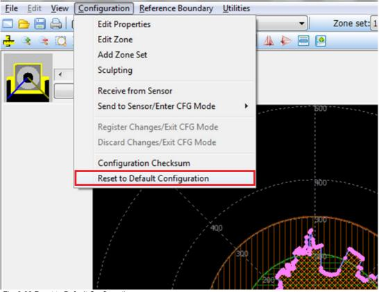
Fig. 3-93 Reset to Default Configuration
