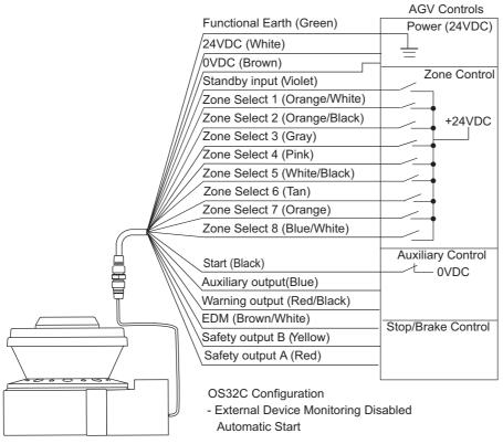
Fig. 5-4 Connecting to AGV Controls
