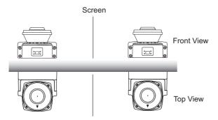
Fig. 4-4 Separation using a screen
