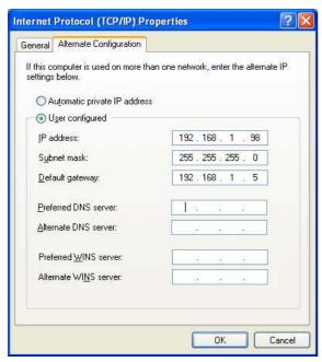
Fig. 3-10 Alternate Configuration
