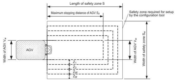
Fig. 4-17 Installation on AGV
