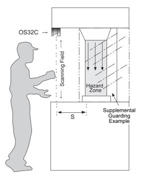
Fig. 4-11 Hand Detection Protection
