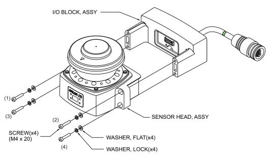
Fig. 7-9 Sensor Block Replacement
