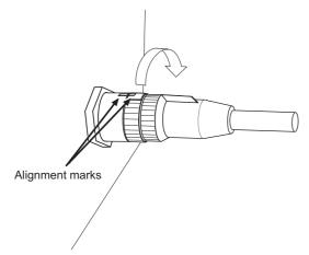
Fig. 4-40 Aligning the XS5 Plug
