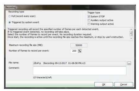
Fig. 3-80 Event Triggered Recording
