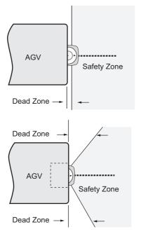
Fig. 4-14 Installation with Bodywork of AGV
