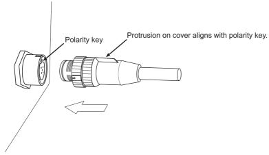
Fig. 4-38 Aligning to polarity key
