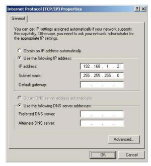
Fig. 3-9 TCP/IP Properties
