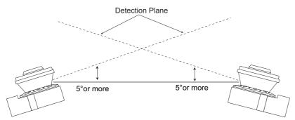
Fig. 4-2 Offset Scanning Level by Tilting
