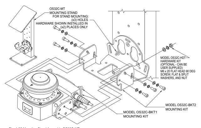
Fig. 4-35 Mounting Stand Assembly OS32C-MT
