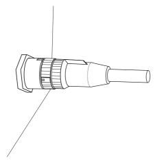
Fig. 4-39 Inserting into the socket
