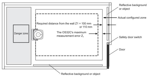
Fig. 7-5 Installing Door on Entrance
