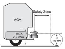
Fig. 4-12 Installation on Automated Guided Vehicle
