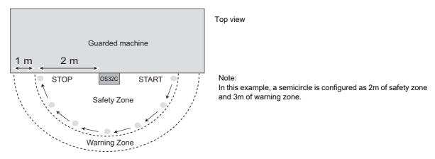
Fig. 6-1 Testing a Horizontal Safety Zone
