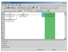
13. Double-click in the rung comment area to write rung comments for the ladder program. It is also possible to write comments by first using either the mouse or the cursor keys to move to the rung comment area, and then selecting *Edit(E)/Edit rung comments*.
