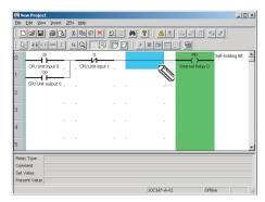
Use the Edit Input Dialog Box to insert a input at the connection line.
