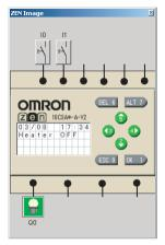
Multiple display bits (D) can be executed simultaneously, and their display conditions monitored.
