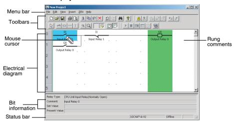
Note To switch between the ladder diagram and electrical diagram displays, either click on the buttons in the Toolbar or else select View(V)/Circuit display method/Ladder rung diagram/ Electrical circuit diagram from the File menu.
