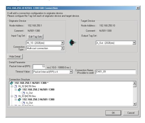
Input 10 ms as the new RPI value in the Edit Connection Dialog Box, and click the **OK** Button. The usage rate of allowable tag data link bandwidth for the device 192.168.250.1 increases to 50.17% as shown in the Usage of Capacity column, and this indicates that the RPI for the specific connection is set shorter.
