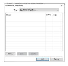
4 Select Input Only (Tag type) or Input & Output (Tag type) from Type and click the New Button.
