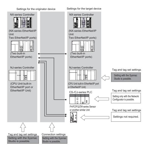
Use the Network Configurator if a CS/CJ-series PLC operates as the originator device.
