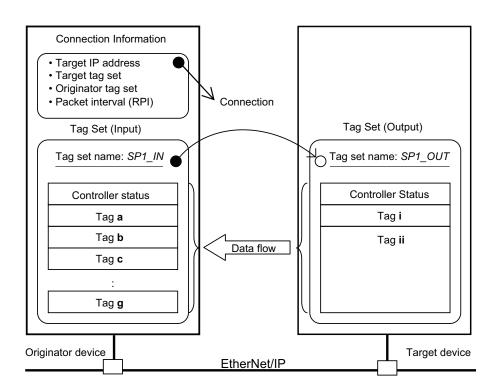
**Note** In this example, a connection is established with the originator's tag list with tags a to g (inputs), which are in a tag set called *SP1\_IN*, and the target's tag list with tags i and ii (outputs), which are in a tag set called *SP1\_OUT*.
