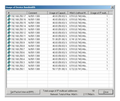
Note that the usage rate of allowable tag data link bandwidth for the device, 192.168.250.10, is also increased from 40.83% to 51.00%.
