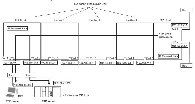
When the CPU Unit executes the FTP client instruction specifying PC1 with IP address 192.168.40.200, an IP packet is transferred to PC1, which is the FTP server, via the EtherNet/IP port 1 on the NX-series EtherNet/IP Unit with unit number 4 in the same network segment.
