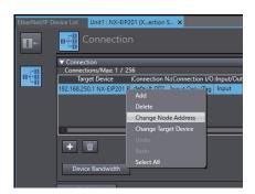
The Node Address Change Dialog Box is displayed. Enter a new IP address in New IP address.
