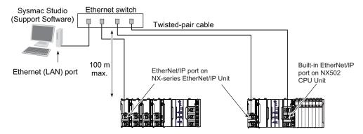
EtherNet/IP System Configuration Example
