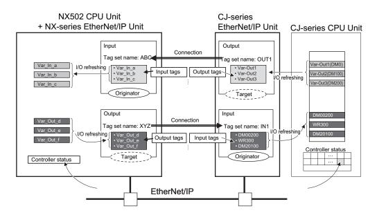
For communications between Controllers, the connection information is set in the EtherNet/IP port of the Controller that receives (consumes) the data (i.e., the originator).
