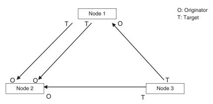
If multicast is specified for data transmission and the node sends out just one multicast packet to other nodes, it requires respective connections for them.
