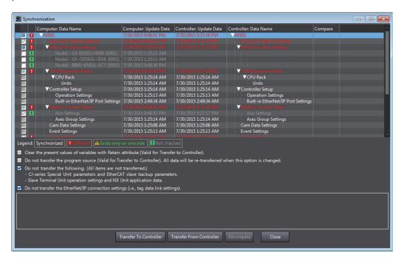
Glear the Do not transfer the EtherNet/IP connection settings (i.e., tag data link settings)
