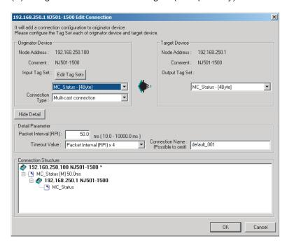
• (B) Using Other EtherNet/IP Devices as Targets (for Settings Other Than Input Only)
