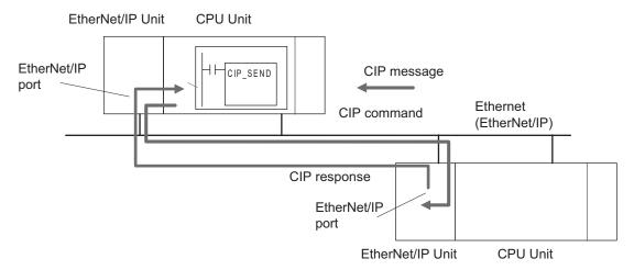
By specifying a route path, you can send CIP messages (CIP commands and responses) to a device on another CIP-based network segment (CIP routing function for message communications). However, since the starting point of route path is the CPU Unit, it is necessary to set the route path that starts from the CPU Unit and passes through the NX-series EtherNet/IP Unit.
