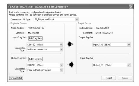
The **Connection I/O Type** list box in the upper part of the **Edit Connection** Dialog Box lists connection I/O types. Select a connection I/O type according to your application.
