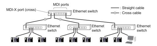
• Some Ethernet switches can automatically distinguish between MDI and MDI-X. When this kind of Ethernet switch is used, straight cable can be used between Ethernet switches.
