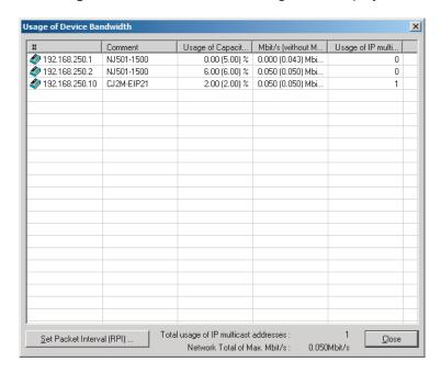
The **Usage of Capacity (without Multicast Filter)** column shows the usage rate of allowable tag data link bandwidth, and the **Mbit/s (without Multicast Filter)** column shows the network bandwidth usage.
