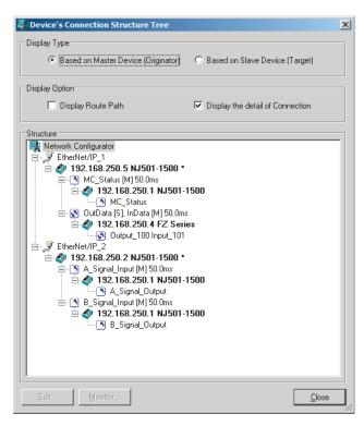
**5** Use the device connection structure tree to change the RPI and timeout settings if necessary.
