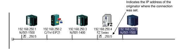
**3** Repeat the connections setting procedure until all of the connections are set.
