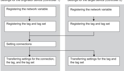
Settings for the originator device (Controller 1) Settings for the target device (Controller 2)
