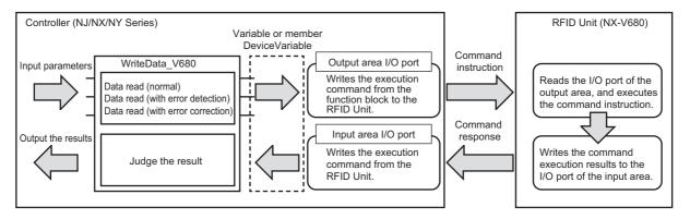
When Execute changes to TRUE, the data of the byte array specified in WriteData is written to the memory of the RF Tag.
