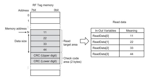
• If *ReadKind* is executed as *With error correction*, the data and check code are read from the RF Tag, and errors in the data are detected, and 1-bit errors are corrected. When using this function, write beforehand the data and check code in the target area as *With error correction* of the function block "WriteData\_V680".
