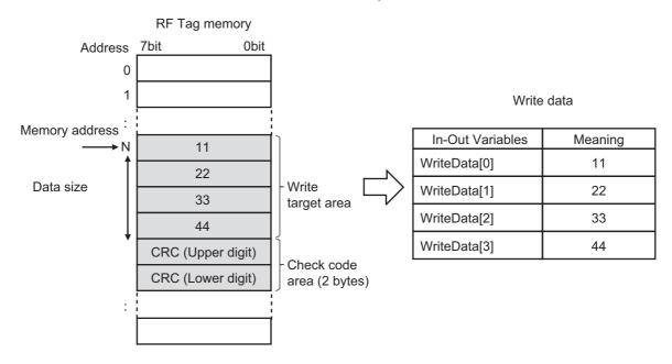
• If WriteKind is executed as With error correction, data is written to the RF Tag target area, and the check code for error correction is written to the last five bytes of the area.
