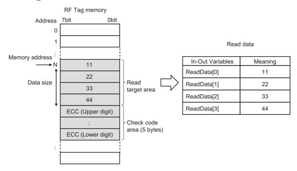
Note If the data and check code are not written beforehand in the target area as *With error detection* and *With error correction* of the function block "WriteData\_V680" when *ReadKind* is executed as "With error detection", a communications error (RF Tag Data Error Detected) will occur.
