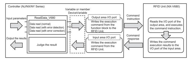
When Execute changes to TRUE, the data read from the memory of the RF Tag is saved to the byte array specified by ReadData.
