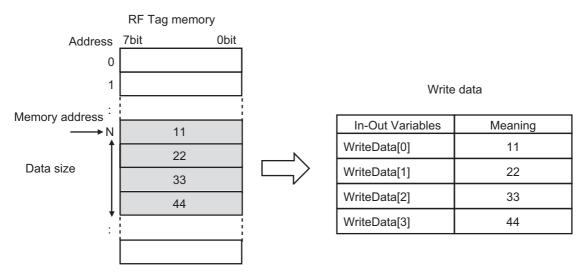
• The memory capacity written to the RF Tag in a single execution varies depending on the specified WriteKind. The values that can be specified in MemoryAddr and DataSize are described below.
