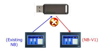
You need to back the existing project data used in the NB to a USB stick memory before replacing your HMI. Then, convert the data with NB-Designer V1.60 or higher to reuse.
