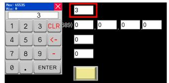
3. After entering 3 for the PLC No.0 then confirming it, the IP address, port number, and node ID set to the host are displayed.
