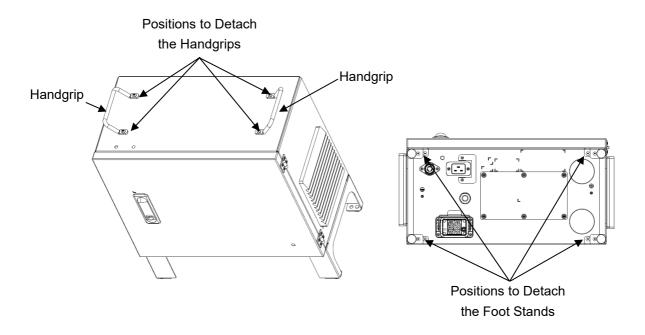
2. Use the screws from the handgrips and the foot stands to mount the brackets on the control box. Note that Foot Stand Brackets for HW3.X and HW5.0 are different.
