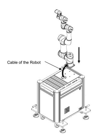
3. Pass the cable of the robot through the cord hole, connect to the control box, and cover the cord hole with a desktop cover.
