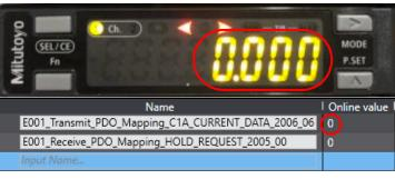
Push and secure the gage head of the Linear Gage. Check that the numerical value (current value) on the "Numerical and indicator display screen" of the Linear Gage is changed.
