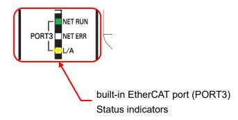
**2** Check the LEDs on the EJ Counter.
