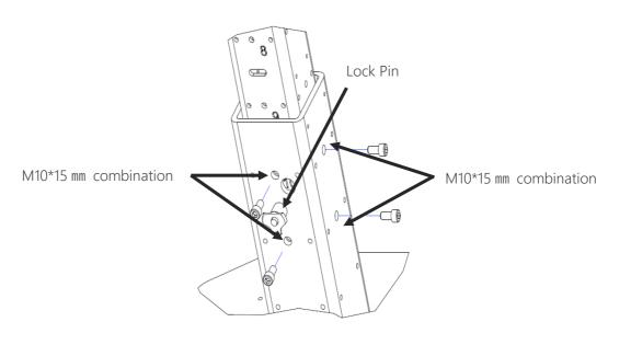
When adjusting the height of the TM Robot Stand, there must be two operators to avoid danger. One helps hold the inner tube, and the other changes the extent. The Corporation will not be liable for any injuries caused during operation.
