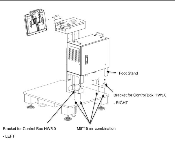
HW5.0 Robot Stick and its holder should be installed properly by the integrated applications or outside the safeguarded space based on the risk assessment. The distance of screw holes is 95 mm with M4\*5 mm screws
