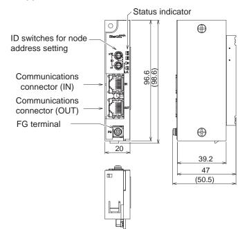
For the overall depth when the EtherCAT Communication Unit is installed with an EtherCAT cable connected, add 76.2 mm to the dimension D of the Inverter. The dimension D differs depending on its capacity of the Inverter. Please refer to the manual for the Inverter.
