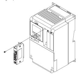
4. Prepare an FG wire and wire it to a grounding location as close as possible to the FG terminal of the Communication Unit. FG terminal screw: M3 x 8 Tightening torque: 0.6 to 0.8 N·m
