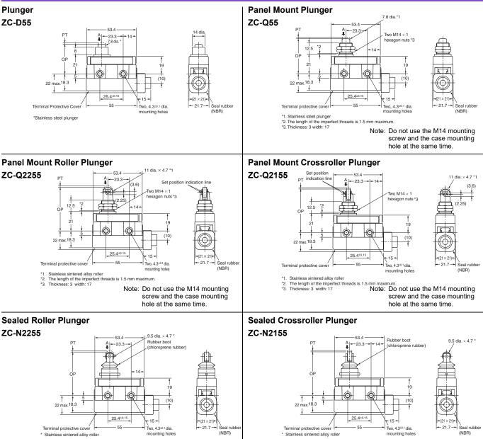
Note: 1. Unless otherwise specified, a tolerance of  $\pm 0.4$  mm applies to all dimensions. 2. Operating characteristics are for when the Switch is operated from direction A.
