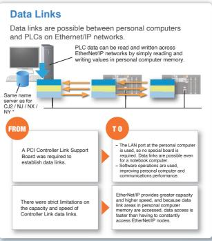
Note: The Network Configurator included in the CX-One Package or Sysmac Studio is required to set tag data links.
