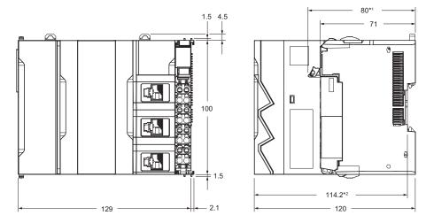
\*1. The dimension from the terminal block lock lever to the back surface of the CPU Unit.
