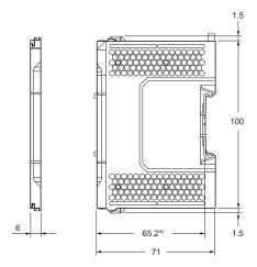
\*1. The dimension from the attachment surface of the DIN Track to the front surface of the end cover.
