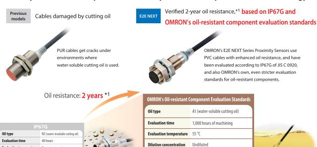
■ Two years\*1 of stable operation verified for pre-wired connector models as well, using similar oil resistance tests
