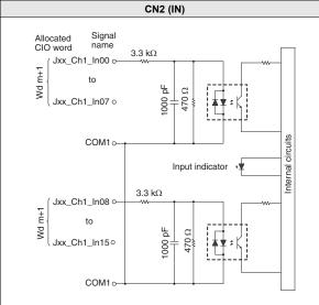
The signal names of the terminals are the device variable names.
