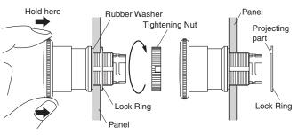
1. When the panel cutout dimension is 25 dia., remove the supplied rubber washer and mount the 25-dia. Ring as shown below. (Since the A22Z-R25 is not attached to the main body, order separately.) When using a Legend Plate (Order Separately), do not remove the rubber washer.
