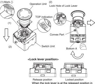
this Switch, the NO and NC contact operation is Set the lock lever to the locked position when us-
