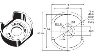
Note: 1. The dimensions of the Shroud conform to the specifications of the SEMATECH Application Guide for SEMI S2-93.
