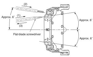
The wiring and screwdriver angles for the Lighting Unit and Switch Block (2 contacts) are the same as for the Switch Block (1 contact) shown in the above illustration.
