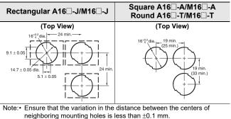
Make sure the thickness of the mounting panel is between 0.5 and 3.2 mm. If, however, a Switch Guard or Dust Cover is used, the thickness of the mounting panel much be between 0.5 and 2 mm
