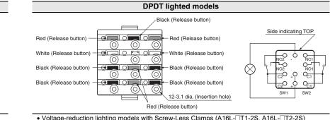
Voltage-reduction lighting models with Screw-Less Clamps (A16L-□T1-2S, A16L-□T2-2S) incorporate voltage-reduction circuits.
