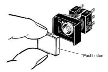
(2) When mounting the Operation Unit to the Case, press the entire surface of the Operation Unit to surface A of the Case as shown in the following diagram.
