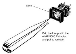
(2) Removing from the Switch End The Lamp can be removed by hand once the Switch is removed using the A16Z-5080 Extractor.
