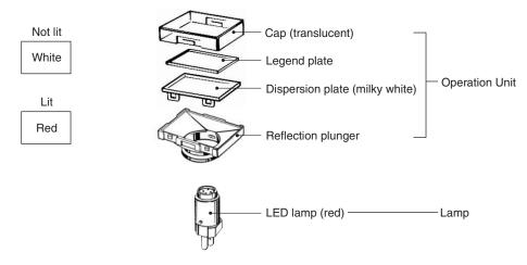
Ordering: For colored illumination, order the Pushbutton, Case, Lamp, and Switch separately.
