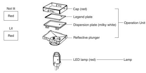
With colored illumination, the color of the lighted surface is white when the LED is not lit and the LED emits another color when it is lit. Example: Red Illumination
