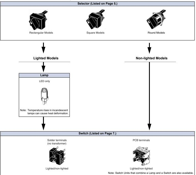
Ordering Individually ....... Selectors, Lamps, and Switches (Sockets) can be ordered separately. Combinations that are not available as sets can be created using individual Units. Also, store the parts as spares for maintenance and repairs. Selectors (Oil-resistant IP65 Models Only)
