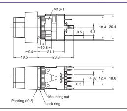
Rectangular A165W□-T Reduced-voltage lighting solder terminals (tab terminals #110)
