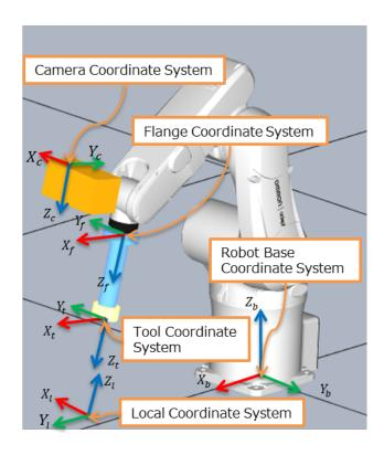
The orientation of the coordinate axes of each coordinate system depends on the robot. Please refer to the instruction manual for each robot.
