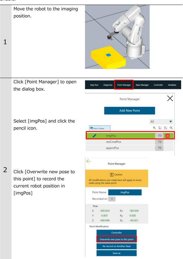
Click [X] to close the Point  $\times$ Point Manager Manager dialog. Add New Point žį Žį Gį TO > imgPos At the [imgPos] point node, the robot moves to the imgPos imaging position. Point Node **WARNING** 3 • These operations drive the robot. • Operate the robot in the state whereby pressing the [Emergency stop] button can stop its motion anytime. In the base list, select [RobotBase] as the current base. In the tool list, select [NOTOOL] as the current tool. 0 RobotBa 🔻 0 NOTOO
