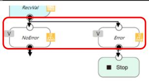
proceed to the next node. Check the TJG of the Vision V Sensor measurement result. g\_FHRobotVision\_O MRON\_param[0] The TJG of the Vision Sensor measurement result is stored in the global variable Stop 3 [g\_FHRobotVision\_OMRON\_pa ram[0]]. If TJG is OK (1), proceed to the next node, otherwise exit the program.
