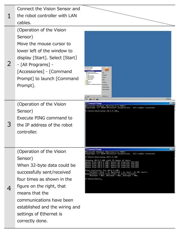
When 32-byte data cannot be sent/received four times and PING command timed out, check whether or not the robot controller is turned on, the wiring was correctly done, or communication settings are correct.
