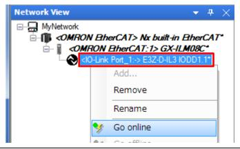
13 Check that Photoelectric Sensor is connected online.
