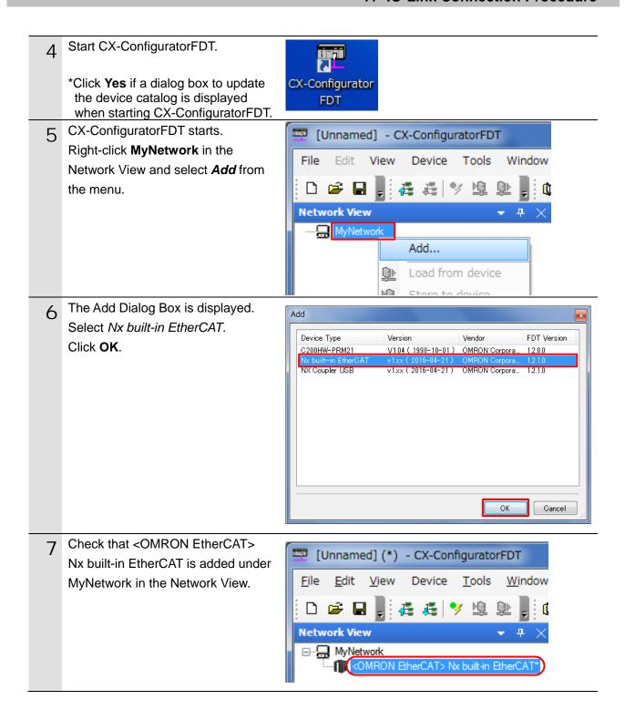
Right-click **<OMRON EtherCAT>**Nx built-in EtherCAT and select
