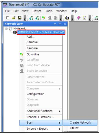
The Lifelist Dialog Box is displayed after completing the network scan. Check that <OMRON EtherCAT:1> GX-ILM08C is added under Nx built-in EtherCAT.
