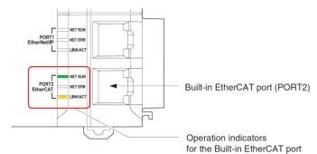
2 Check the LED indicators on IO-Link Master Unit.
