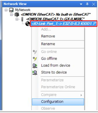
14 The <IO-Link Port\_1:-> E3Z-D-IL3 IODD1.1 - Configuration Tab Page is displayed.
