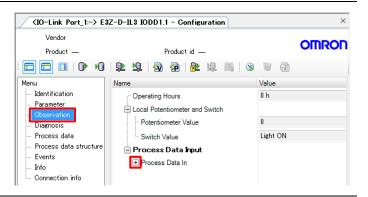
16 Click the ☑ icon (Enable or disable cyclic read from device for dynamic variables) on the <IO-Link Port\_1:-> E3Z-D-IL3 IODD1.1 - Configuration Tab Page.
