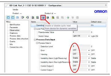
17 Check that Operation mode switch on Photoelectric Sensor is set to Light ON (factory setting).
