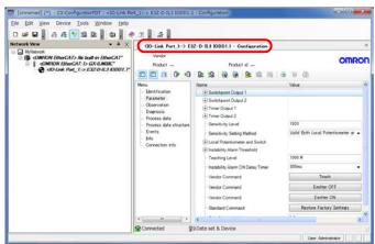
15 Select **Observation** listed under Menu on the <IO-Link Port\_1:-> E3Z-D-IL3 IODD1.1 - Configuration Tab Page.
