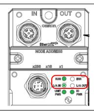
3 Check the I/O indicator for Port 1 on IO-Link Master Unit.
