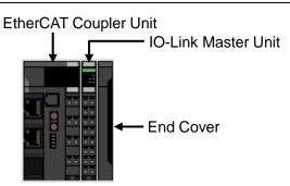
3 Check the position of the hardware switches on EtherCAT Coupler Unit by referring to the figure on the right.
