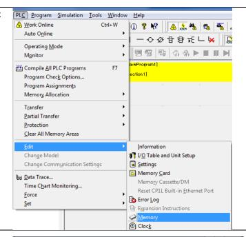
3 The PLC Memory Window is displayed. Double-click **D** on the Memory Tab of the PLC Memory Window.
