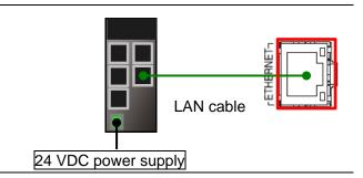
6 Connect 24 VDC power supply to 24 V input terminal block.
