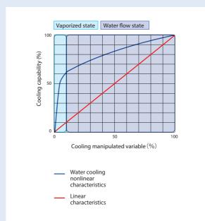
It constantly detects changes in the temperature behavior and suppresses the temperature variation by automatically adjusting the proportional band (cooling).
