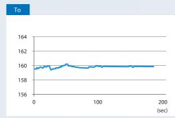
When the automatic filter adjustment function of the E5  $\square$  D /NX-TC is used, this periodic temperature variation is suppressed automatically. It becomes possible to perform stable temperature
