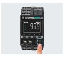
"MANU MEAS" switch on the lower right of the front panel
