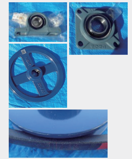
Correct positioning of belt and pulley
