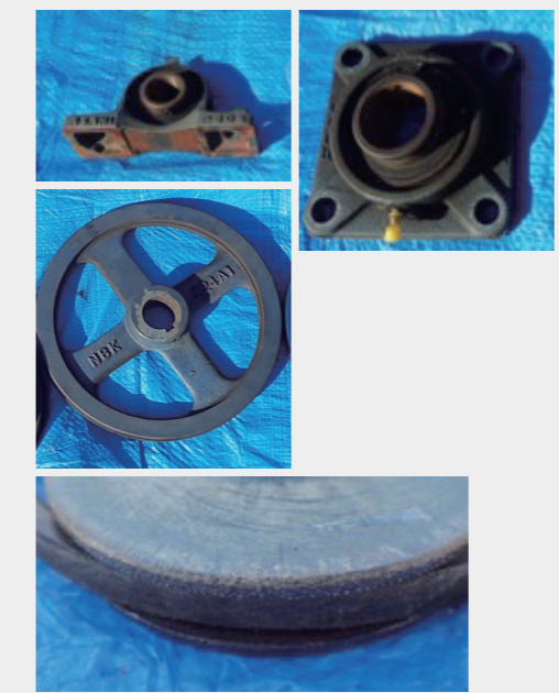
Belt and pulley worn down by friction
