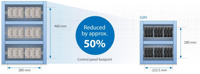
Example: Installation of 18 SSRs configured for three-phase heaters (6 channels)
