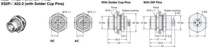
Front Lock Model XS2P-D522-1 (with DIP Pins) XS2P-D522-2 (with Solder Cup Pins)
