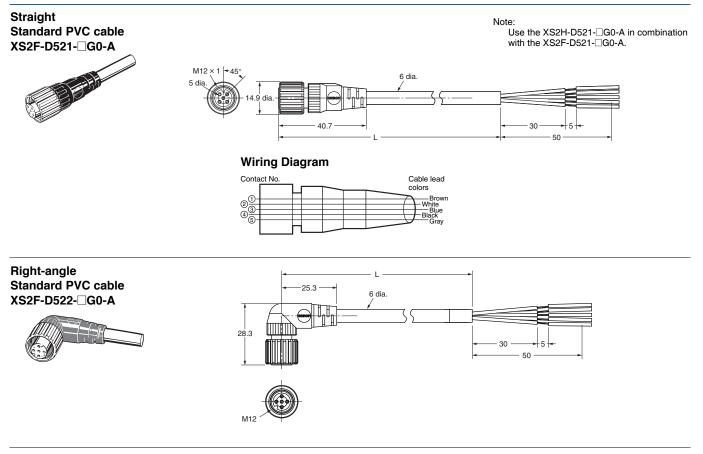
For details on connecting with E2E Proximity Sensors, refer to E2E Small-diameter Proximity Sensor Data Sheet (Cat. No.: SCEC-044).
