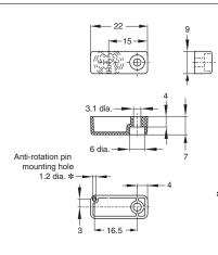
\* D41D-A3 mounting hole is fixed in place with an M3 screw. The actuator can be prevented from twisting caused by screw tightening torque during installation by passing a pin up to 1.1 mm in size through the hole in the rear section of the D41D-A3.
