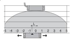
5 mm misalignment tolerance after setting
