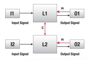
Category 4 systems use two channels as well (homogenous or divers). Monitoring (m) and cross-monitoring (C) is used to detect multiple failures in the system without loosing the safety function.
