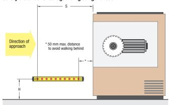
The height of the protective field "H" above the reference plane and the resolution "d" of the safety sensor system have the following relationship:
