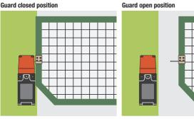
By means of a separated actuator the switch is automatically activated.
