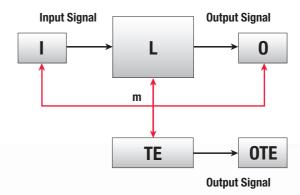
This example shows a category 2 system with two separate outputs. The Test equipment (TE) monitors (m) the correct function of the Input, Logic and Output. If the test results are ok, the test output (OTE) is activated. A failure in the safety system can be detected by the Test equipment and will not result in a loss of the safety function since the shutdown still can be done via the second channel.
