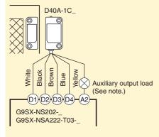
Note: The auxiliary output load current must be 10 mA max.
