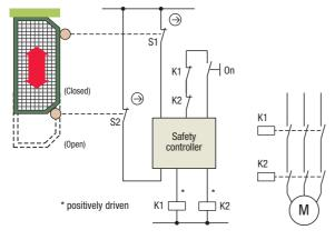
Redundant Safety Limit Switches or Safety Door Switches are used to Safety Input: monitor the position of the guard.
