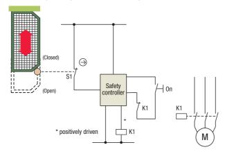
Safety Input: A Safety Limit Switch or a Safety Door Switch is used to monitor the position of the guard.
