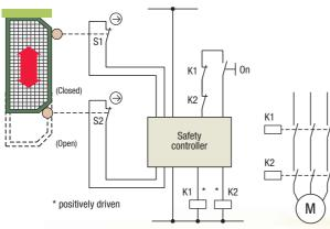
Safety Input: Redundant Safety Limit Switches or Safety Door Switches are used to monitor the position of the guard. Separate in- and outputs for the switches enable the Safety Control to detect cross connections
