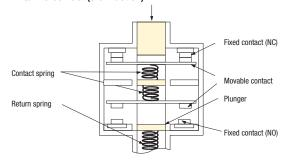
NC contacts conform to EN60947-5-1 Direct Opening
