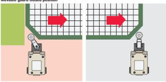
Wrong: Switch is not automatically activated when opening the safety devices.
