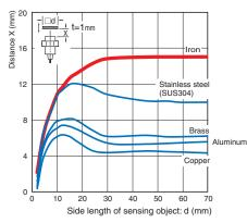
Double distance model, Spatter-resistant Double distance model | Single distance model, Spatter-resistant Single distance model Size: M8 E2E(Q)-X1R5 8
