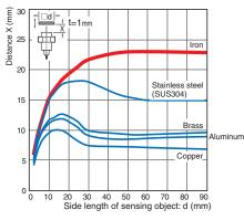
Triple distance model, Spatter-resistant Triple distance model Size: M8 E2E(Q)-X3□8
