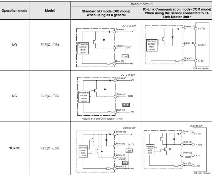
\* In the IO-Link mode, the cord between the IO-Link master and sensor must have a length of 20 m or less.
