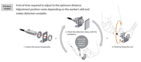
3. Loosen the nut and adjust the distance.
