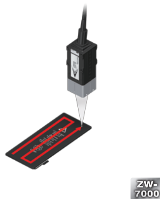
Flatness measurement of batteries
