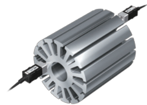
Thickness measurement of motor cores
